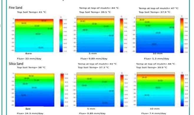
Figure 4. Shows the temperature profile of the sand columns using different types of sandy soil and SHS mulch thicknesses
