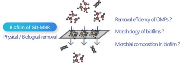
In this study, three different conditions for the GD-MBRs were tested with real wastewater : no-aeration (NA), continuous aeration (CA), and intermittent aeration (IA). Diclofenac (DCF), Carbamazepine (CBZ), and sulfamethoxazole (SMX) have been selected due to their widespread usage. GD-MBR operated without OMPs for 78 days to grow the biofilms, and selected OMPs are dosed for 28 days.
