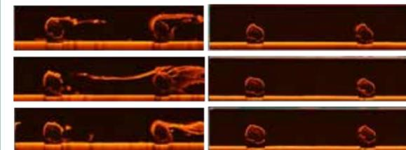
Fig 3: Spatial biofilm distribution on coated and uncoated feed spacer surfaces at the end of study
