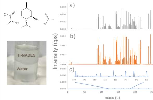
Figure: left H-NADES components, and H-NADES:WATERS two phase solution; right: HR-ICP-MS spectrum of a multielement solution with a concentration of 10 ppm before contact with H-NADES (a), after contact with H-NADES M:A(b) and M:LA(c).
