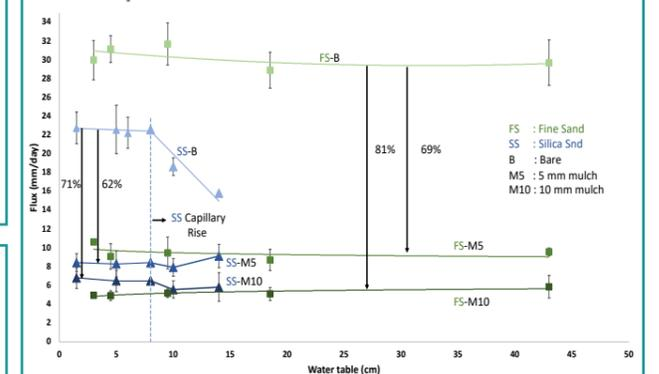
Figure 3. Experimental evaporative fluxes as a function of water table depth for 5 and 10 mm-thick SHS layers.
