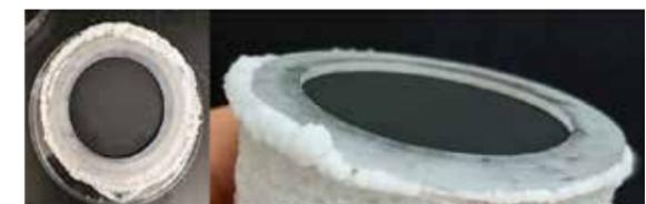
Salt harvesting around the membrane. The photothermal layer remained intact.
