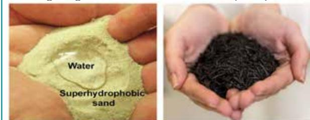
Fig 1. Superhydrophobic sand(left) and biochar(right)
