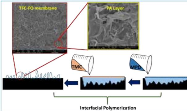
Fig. 2. Fabrication of polyamide (PA) layer on the as-prepared PAN nanofiber substrate using interfacial polymerization.
