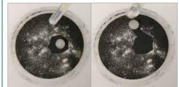
Self-cleaning properties of the superhydrophobic photothermal layer
