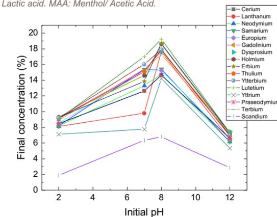
Figure 2: Final concentration of REE, detected by HR ICP-MS, on fresh water after extraction with NADES at different pHs
