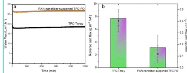
Fig. 3. Performance comparison of the as-prepared TFC-FO membrane and commercial membrane (TFC-Toray) (a) Water flux and (b) reverse salt flux and specific salt flux. AL-FS mode, Draw solution and feed solution are 0.5M NaCl and DI, respectively.
