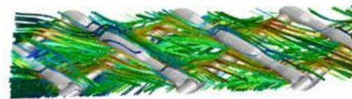
Flow patterns in the feed and permeate channels
