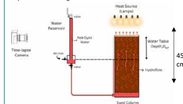
Figure 1. A schematic of the experimental rig used to quantify evaporative fluxes from the sand.
