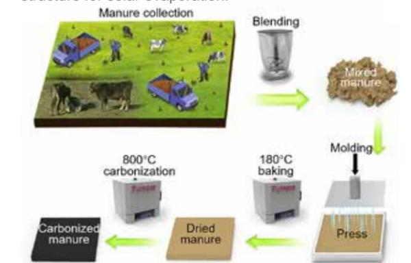
Figure 1: The fabrication process of carbonized manure.
