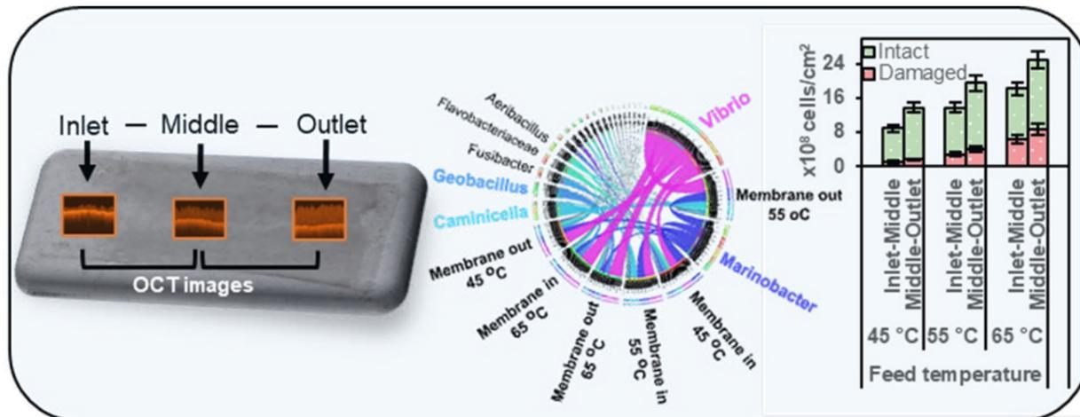
Fig. 1. Analysis of the spatial and temporal biofilm distribution: OCT imaging (left), microbial community analysis (middle), spatial distribution of intact and damaged cells (right) [1].
