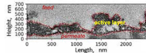
Example of polyamide active layer geometry obtained by TEM. The layer thickness is very irregular, thus a 1D representation is not suitable.
