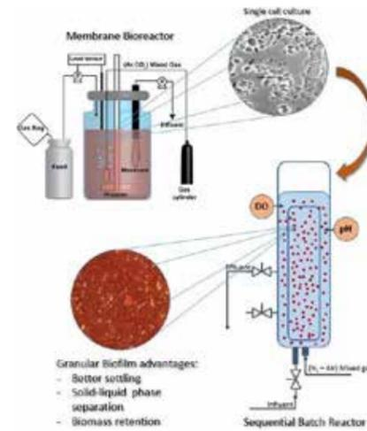
2. Development of a single-stage partial nitrification/anammox process
