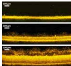
The stabilized permeate flux and effluent quality are directly linked to the formation of porous biofilm layer on the GDM membrane surface, which is the result of the deposition of organic and non-biodegradable substances, and microorganisms. [1]
