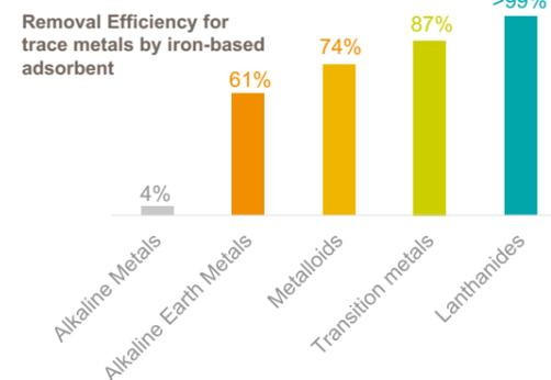
Figure 3: The iron-based adsorbents showed good performance for the removal of Lanthanides, Metalloids and Transition Metals at trace concentrations.
