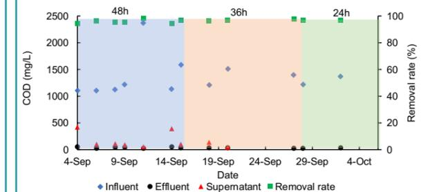
Figure 4. COD removal performance of demo-scale wastewater treatment plant
