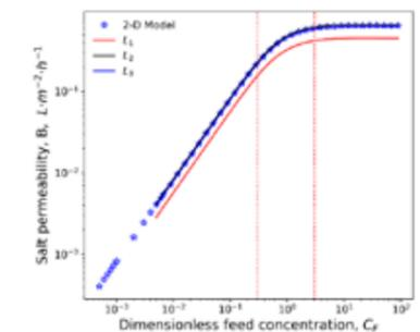
Active layer salt permeability  $B_s$ , function of a dimensionless feed salinity  $C_F$ , computed with the 2D model (blue stars) and with the 1D model using three methods to express equivalent thicknesses.
