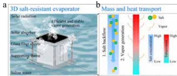
**Figure 1. a.** Schematic of the 3D salt-rejection evaporator, **b.** Working principle includes salt rejection and evaporation enhancement.
