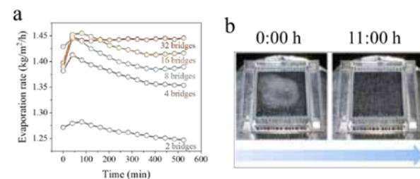
**Figure 2. Salt rejection performance. a.** Evaporation rate variations of evaporators with different MTBs number, **b.** Photos of salt re-dissolving from the surface of a 32-bridge evaporator.
