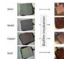
**Figure 3.** Examples of metals used for modifying anodes.
