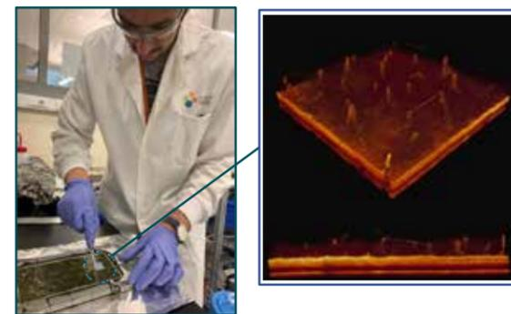
Fig. 3: 3D visualization of OCT scans [3]
