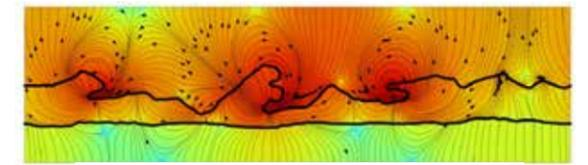
Ionic currents in a charged membrane, as streamlines with direction arrows. Color scale represents the magnitude of ionic current density on a logarithmic scale.
