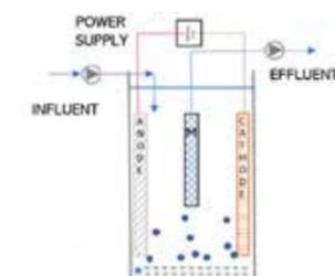
**Figure 4.** Scheme of a bioelectrochemical reactor configuration for this study.
