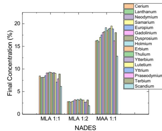
Figure 1: Final concentration of REE, detected by HR ICP-MS, on fresh water after extraction with different NADES at initial pH 2. MLA: Menthol/ Lactic acid. MAA: Menthol/ Acetic Acid.
