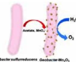
Figure 1. Biohybrid catalyst made with *G. sulfurreducens* and manganese oxide
