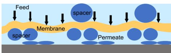
Deformation of feed/permeate spacers and membrane can affect the process performance
