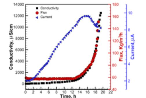
Fig. 3. Changes in DCMD parameters pore wetting induced by a 200 mg/L of sodium dodecyl sulfate.
