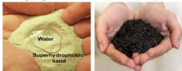
Fig 1. Superhydrophobic sand(left) and biochar(right)
