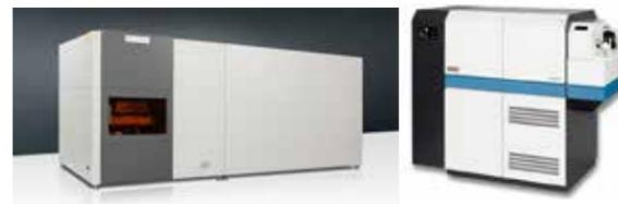
The Element XR HR-ICP-MS coupled ASI J200 Femto QX Tandem laser ablation is able to resolve all of mass overlaps and it can provide lateral resolution of 2 microns.
