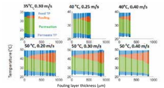
Contributions of each heat transfer resistance in the overall temperature loss, during growing fouling layer thickness. Blue: feed/permeate temperature polarization (top/bottom); Red: temperature drop in fouling layer; Green: temperature drop over the membrane (water vapor flux).
