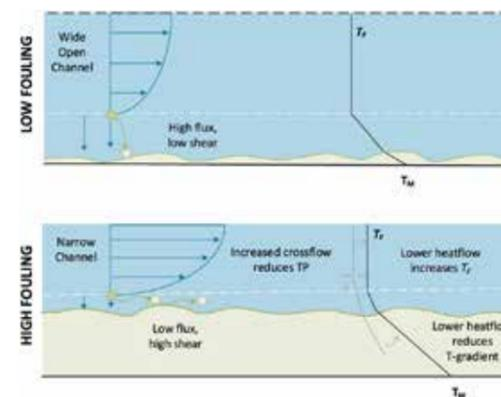
Mechanisms occurring upon fouling layer formation in direct contact membrane distillation: influence of hydrodynamics, temperature profiles and driving forces. Top: clean membrane; Bottom: after cake layer formation.
