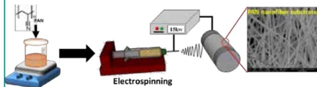
Fig. 1. The fabrication process of PAN nanofiber substrate by electrospinning technique..
