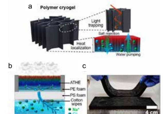
Figure 2: (a) The agar cryogel with vertically aligned light trapping channels efficiently absorbs solar flux. These channels simultaneously serve as water-pumping and salt-dissipation pathways. (b) Polystyrene foam serves as a thermal barrier to reduce heat dissipation towards the bulk seawater. (c) Large-area agar hydrogel evaporator.
