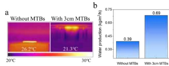
**Figure 3. Boosted water production. a.** Demonstration of the bulk water temperature after 3 h operation with different evaporators, **b.** Water production of evaporators with and without MTBs structure.
