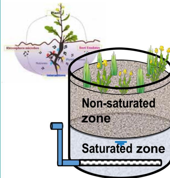
Fig.2 The configuration of the nature-based biofiltration system
